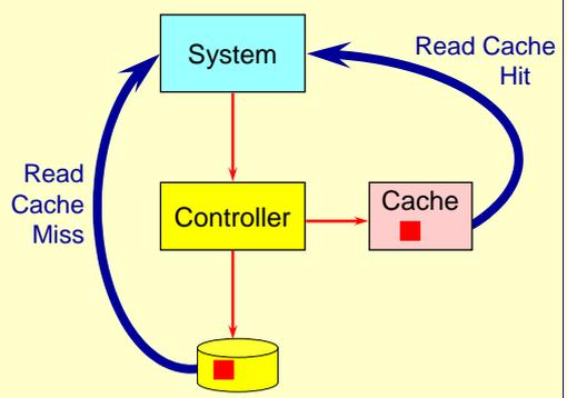
The diagram illustrates the data flow in a controller read cache. A 'System' (light blue box) sends a request to a 'Controller' (yellow box). The Controller is connected to a 'Cache' (pink box) and a disk (yellow cylinder). A red arrow points from the Controller to the Cache. A blue arrow labeled 'Read Cache Hit' loops from the Cache back to the System. A blue arrow labeled 'Read Cache Miss' loops from the Controller to the disk and back to the Controller.
