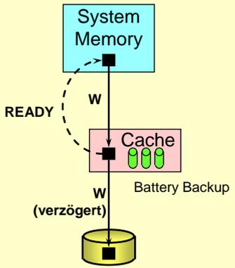
The diagram illustrates the Write Back Cache architecture. It shows a flow from System Memory to a Cache, and then to a storage device. A dashed arrow labeled 'READY' points from the Cache back to System Memory, indicating immediate acknowledgment. A solid arrow labeled 'W' points from System Memory to the Cache. Another solid arrow labeled 'W (verzögert)' points from the Cache to the storage device, indicating a delayed write. The Cache is labeled 'Cache' and 'Battery Backup'.
