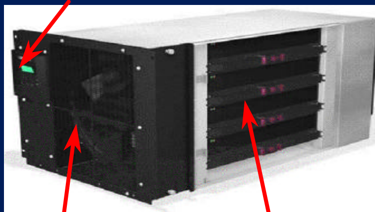
Four dual-processor modules (eight total)
